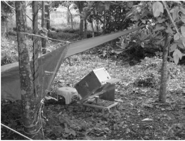
Fig. 1. The microwave radiometer deployed in the field.
