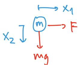
$$m\ddot{\vec{x}} = m \begin{pmatrix} \ddot{x}_1 \\ \ddot{x}_2 \end{pmatrix} = \vec{R} = \begin{pmatrix} F \\ mg \end{pmatrix}$$
