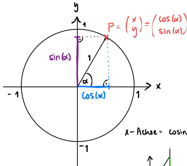
x-Achse = Cosinus, y-Achse = Sinus
