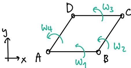
$$\boxed{\omega_1 = \omega_3} \quad \text{und} \quad \boxed{\omega_2 = \omega_4}$$
