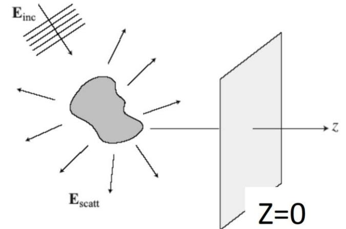
$$\hat{\mathbf{E}}(k_x, k_y; z = \text{const.}) = \frac{1}{4\pi^2} \iint E(x, y; z = \text{const.}) \cdot e^{-i(k_x \cdot x + k_y \cdot y)} dx dy$$
