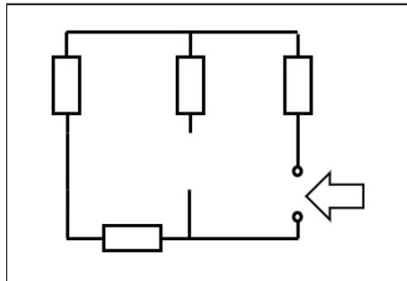
$$\underline{R_i} = 100\Omega + 100\Omega + 100\Omega = \underline{300\Omega}$$
