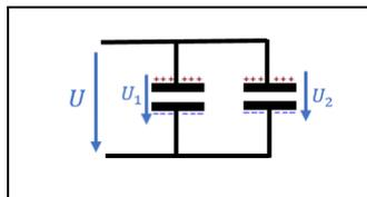
$$\underline{U_1 = U_2 = U} \text{ und } C_1 = \frac{Q_1}{U_1} \rightarrow \underline{Q_1 = C_1 \cdot U}$$
