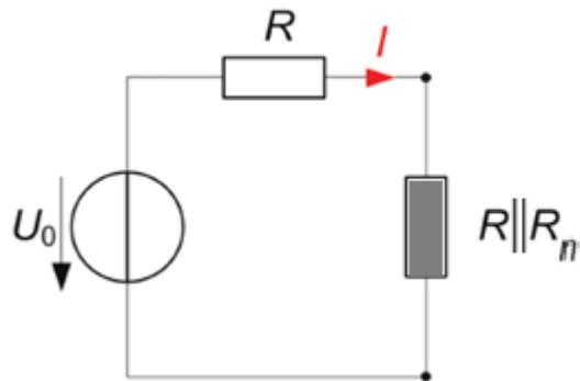
$$\begin{aligned}(R || R_n) &= R \\ \rightarrow R_n &= \infty \\ \rightarrow I_n &= 0\end{aligned}$$
